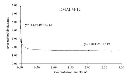
Fig. 7. Critical coalescence concentration (CCC) of DMALM-12
