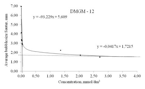
Fig. 6. Critical coalescence concentration (CCC) for DMGM-12
