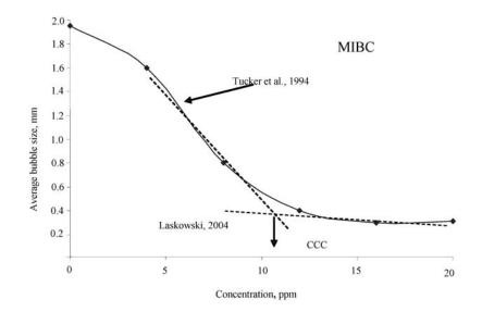
Fig. 1. Influence of concentration frother on properties of the gas-water system for methyl isobuthyl carbinol (MIBC) and CCC determination (Laskowski, 2004; Tucker et al.,1994; Drzymała, 2007)
