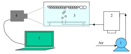
Fig. 4. Experimental set up for CCC measurements: 1) peristaltic pomp, 2) equalizing tank, 3) cell, 4) digital camera, 5) computer (Szyszka, 2006)
