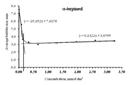
Fig. 2. Critical coalescence concentration (CCC) for  $\alpha$ -terpineol (Szyszka et al., 2006)
