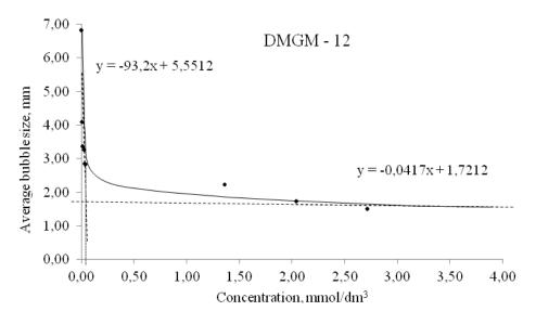
Fig. 5. Critical coalescence concentration (CCC) for DMGM-12
