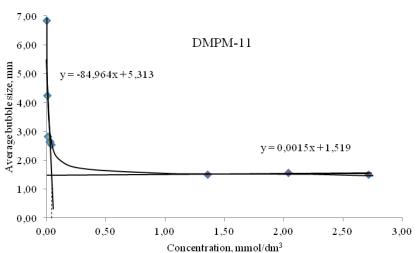
Fig. 9. Critical coalescence concentration (CCC) for DMPM -11
