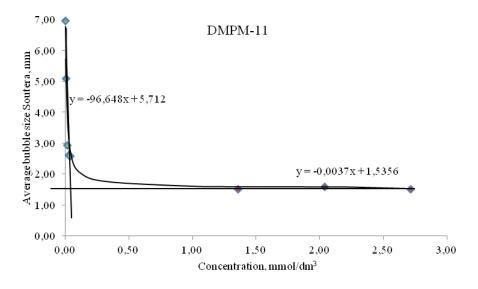
Rys. 10. Critical coalescence concentration (CCC) for DMPM-11
